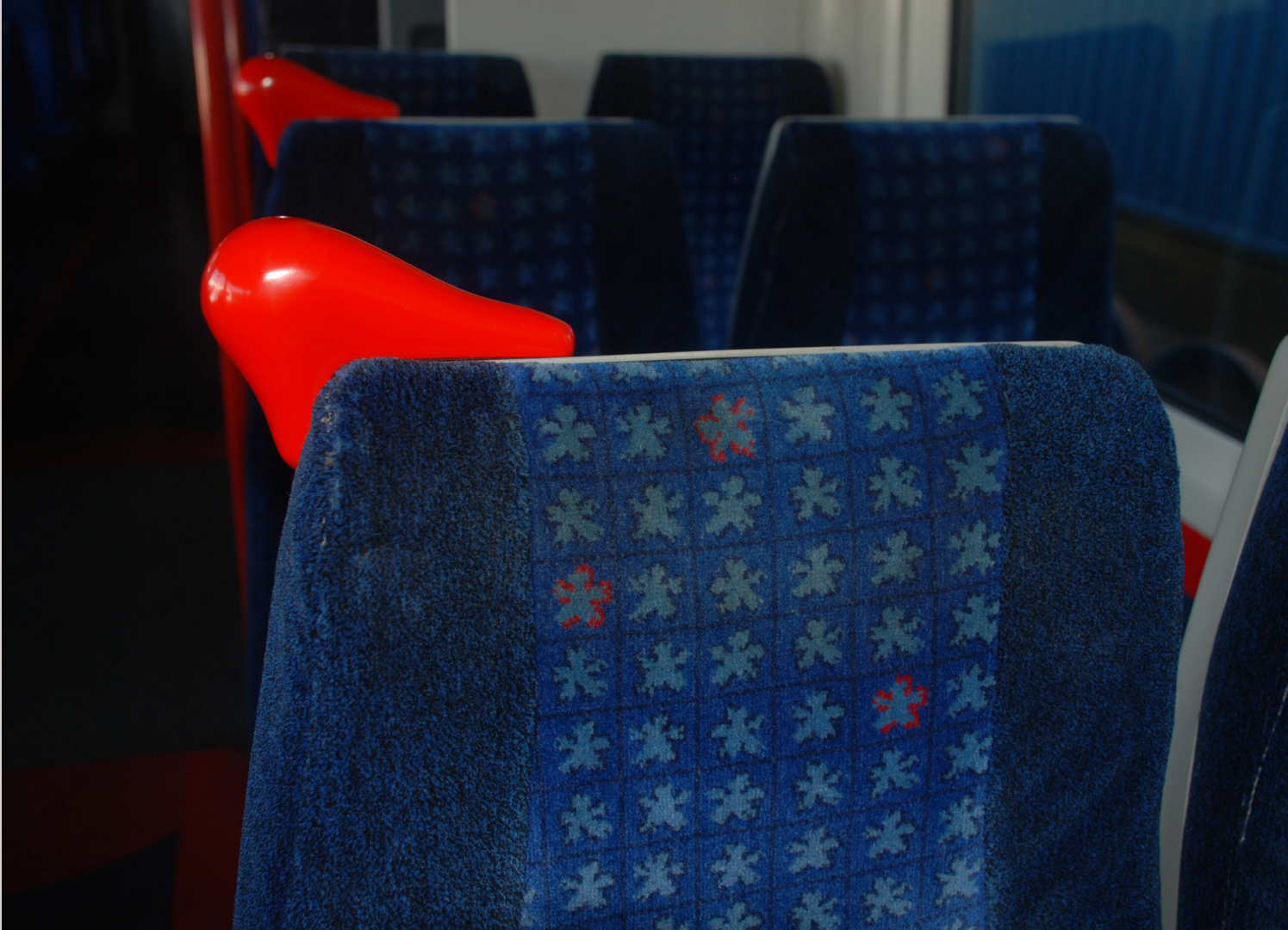
3D printed grab handles installed on a Chiltern Railways train.
