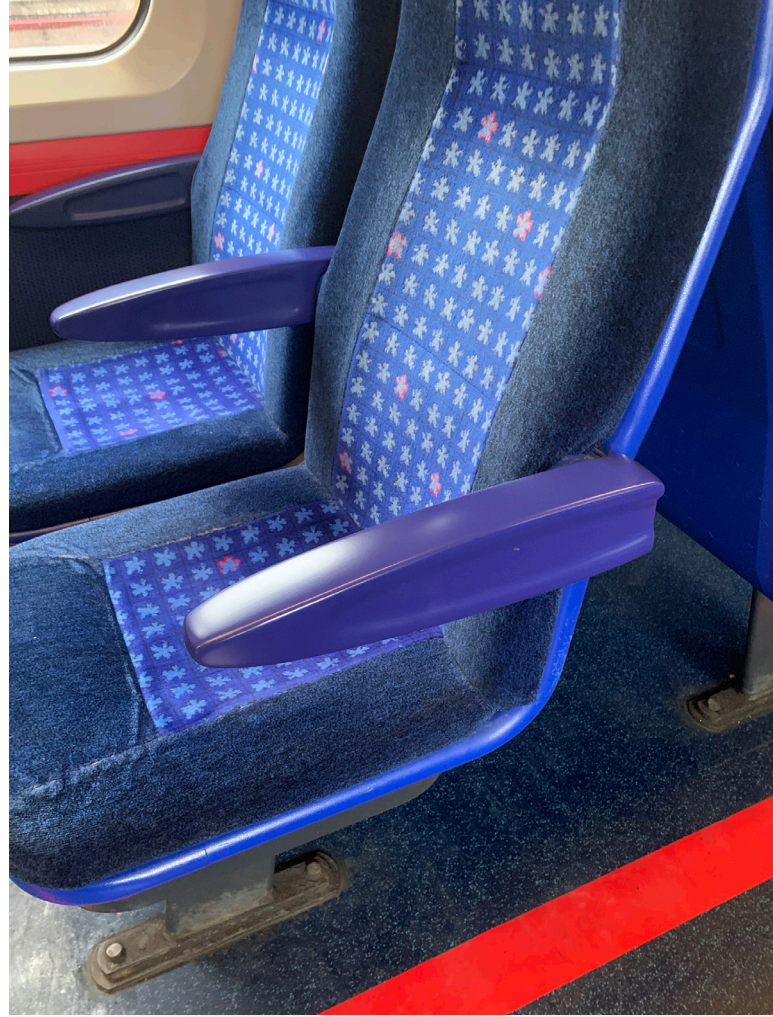
3D printed armrest on Chiltern Railways train – produced 94% faster compared to traditional manufacturing methods.
